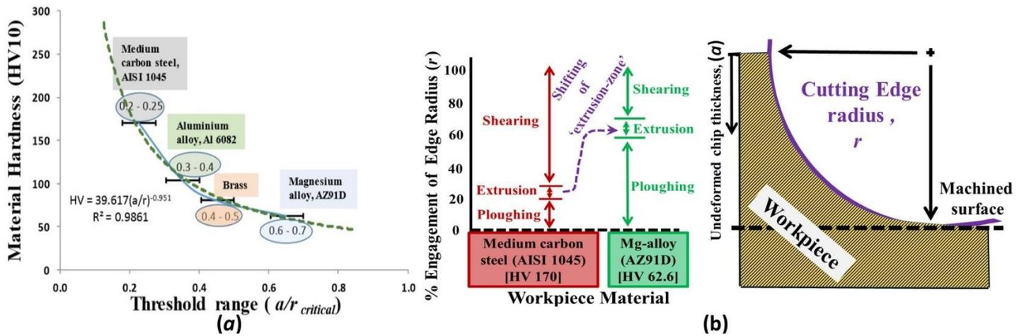
Fig. 3. Illustration of the (a) variation of material hardness with  $a/r$  for achieving 'extrusion-like' finishing (Rahman, Amrun, et al., 2017), (b) Shifting of 'extrusion-like' machining zone for different materials of AISI 1045 and AZ91D as a function of ( $a/r$ ) (M. A. Rahman, M. Rahman, et al., 2018a). Reprinted with permission.
