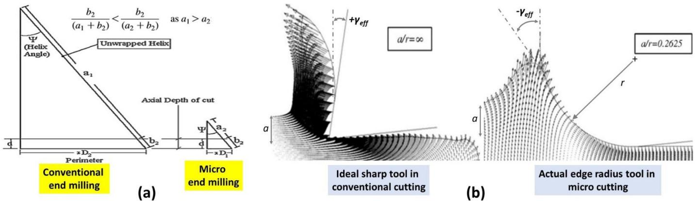
Fig. 2. Illustration of the difference between (a) conventional and micro end milling (Zaman et al., 2006), (b) ideal sharp tool ( $r = 0$ ) in conventional cutting and actual tool with edge radius ( $r$ ) in micro cutting (Woon et al., 2008). Reprinted with permission.
