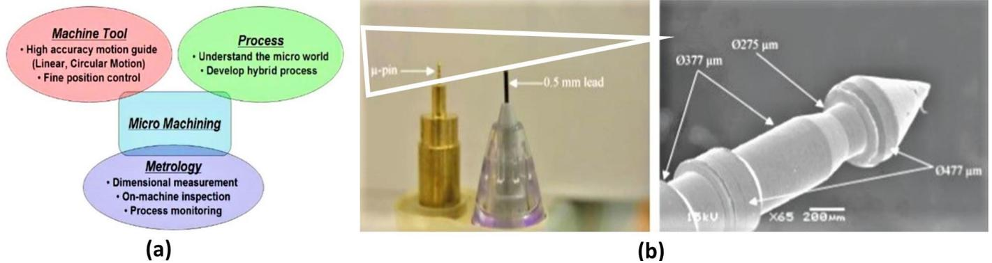
Fig. 1. (a) Collective push on technologies required for micromachining (M Rahman et al., 2010), (b) miniaturized compound shaped pin (Rahman et al., 2005). Reprinted with permission.
